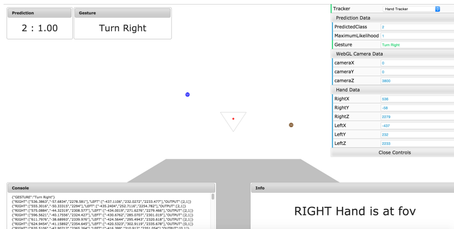
Figure 3.5: Control Center displays received data of hand positions and prediction results
