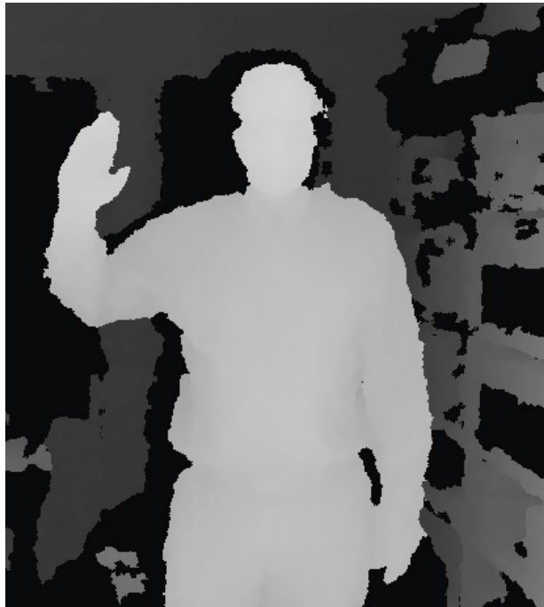
Figure 2.5: Depth Image captured by Asus Xtion PRO LIVE using OpenNI. The darker the color of a pixel, the farther it is from the sensor. [?]
